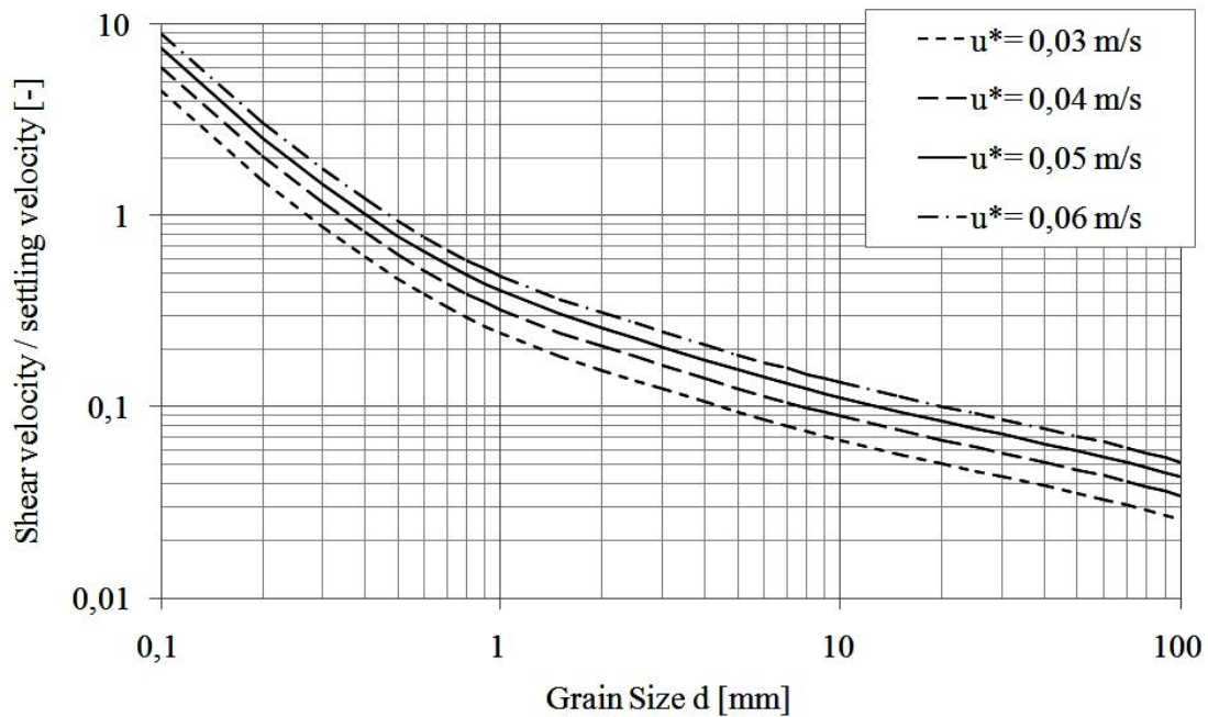
Fig. 5.3 Variation of ratio shear velocity / settling velocity with grain size and shear velocity
