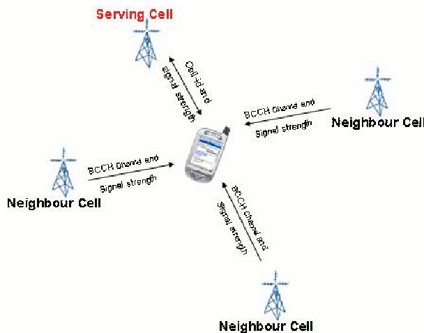
Figure 4: terminal based positioning with the usage of cell-id and neighbour cells
