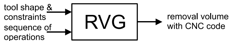
Figure 3-8: Inputs and output of the Manufacturing Removal Volume Grammar (RVG).
