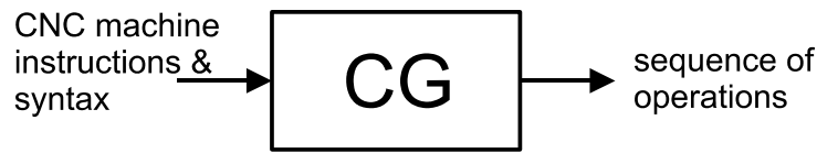
Figure 3-5: Input and Output of the Machine Tool Controller Grammar (CG).
