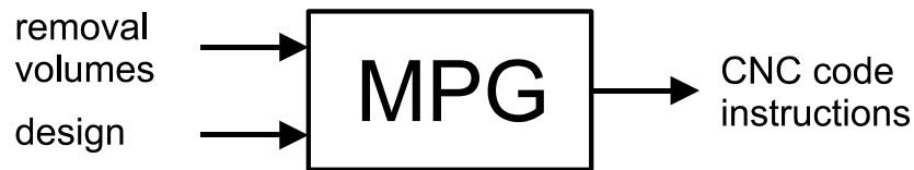
Figure 3-12: Inputs and output of the Mapping Grammar (MPG).
