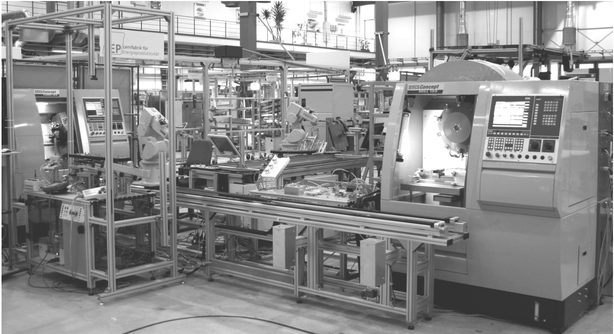
Figure 1-11 Cognitive Machine Shop (CogMaSh) hardware setup.
