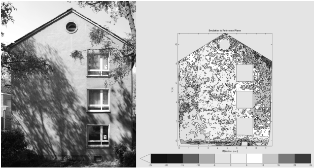
Figure 3: Rectified measuring image (left) and wireframe model with DTM analysis of the façade topography.
