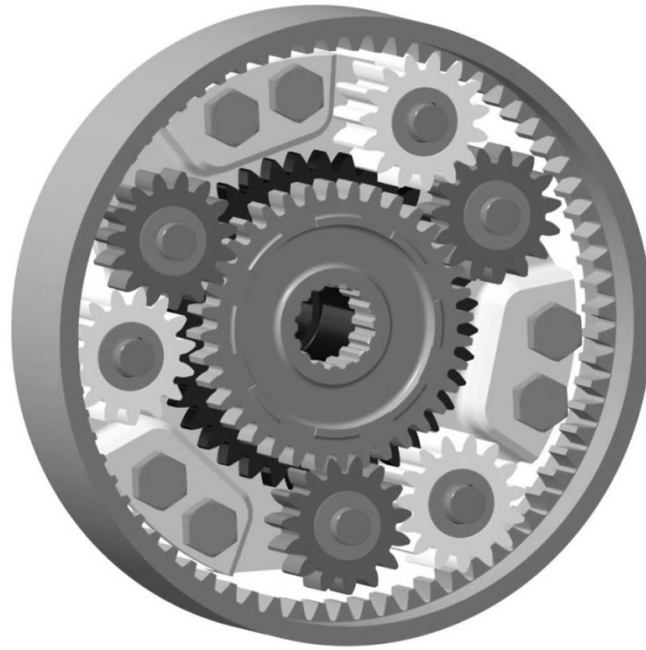
Figure 1-1: Complex-compound planetary gear transmission of the Ravigneaux type [6_RAV38]
