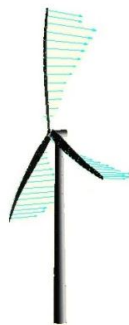
Load distribution during a transient aero-servo-elastic simulation of a 5MW class wind turbine
