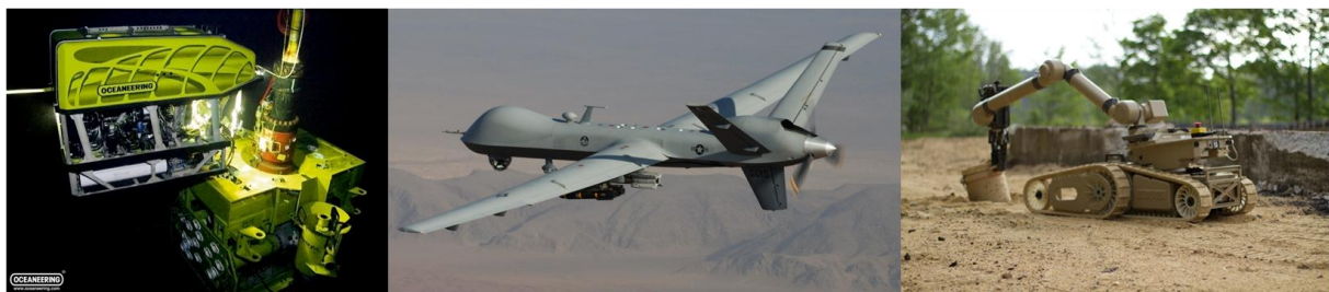
Figure 2-3: Typical representatives of the major mobile telerobotic classes. From left to right: Oceaneering Millennium Plus ROV at work at an undersea oil well [114], General Atomics Reaper UAV [115], iRobot Warrior UGV [116] disarming an IED.
