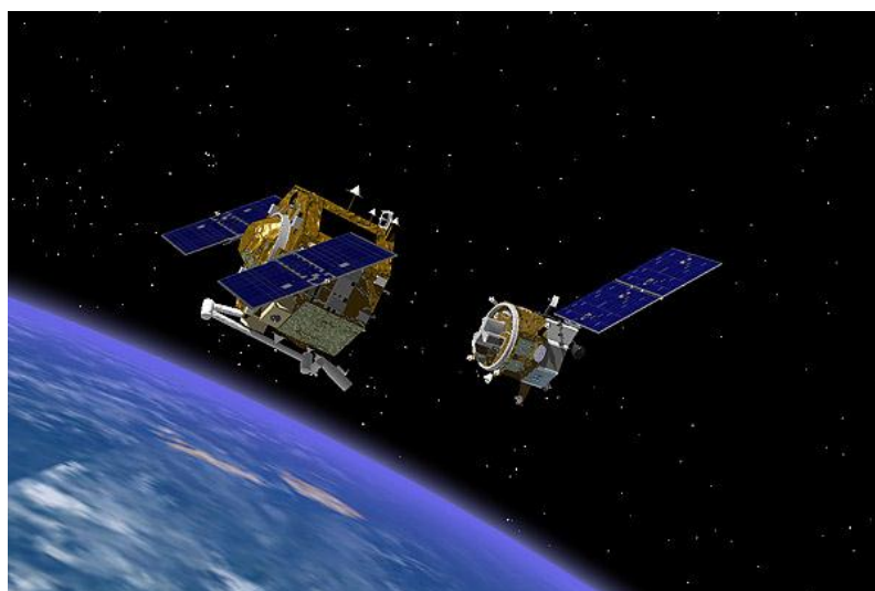
Figure 1-4: Artwork of Orbital Express . ASTRO (left) is approaching NEXTSat with the manipulator in stowed configuration [81]
