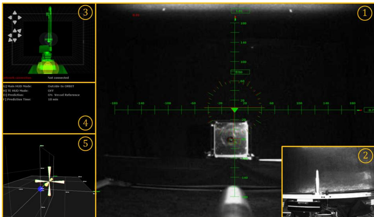
Figure 7-10: Layout of the ThirdEye Proximity Operations GUI . The display functional sections are highlighted. Section 1 contains the main video stream, in this case the chaser primary camera view, and its attitude HUD overlay. Section 2 shows the secondary camera, in this case the ThirdEye view. Section 3 provides the ThirdEye status display and posture prediction. Section 4 contains information about the state and activity of the individual display elements main view attitude HUD, secondary view attitude HUD, prediction display mode, and prediction display propagation time.
