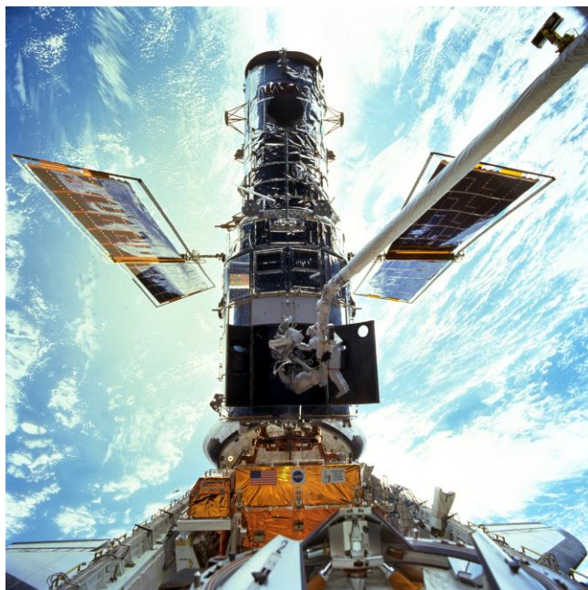
Figure 1-1: Astronauts working on the Hubble Space Telescope fixated in shuttle Discovery's payload bay [69]. Hubble is supported by a rotating table in the payload bay. The RMS supports the astronauts in their repair tasks. This view shows the complex coordination between Shuttle, RMS and astronauts to accomplish servicing missions
