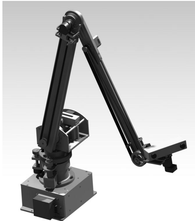
Figure 7-1: CAD model of the ThirdEye robotic camera arm. Note the belt-driven elbow and camera head elevation joints. This design was chosen to reduce the mass of the limbs and thus the motor torque requirements. The CAD model does not show the secondary electronics box which is mounted to the right side of this view.
