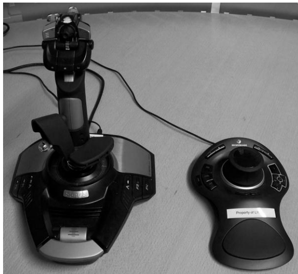
Figure 6-10: Input devices used during the HUD evaluation experiments. The Saitek Cyborg Evo Force joystick is shown to the left, with the 3DConnexion SpaceExplorer 6DOF input device to the right.
