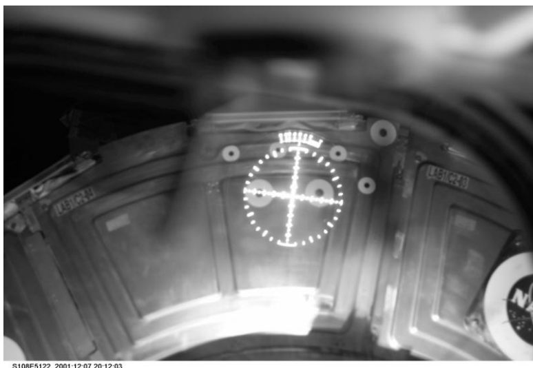
Figure 11-9: COAS during an approach of ISS [192]
