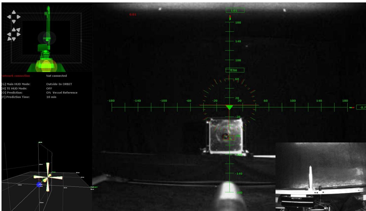
Figure 6-31: Attitude HUD and trajectory prediction display integrated into the ThirdEye proximity operations GUI.
