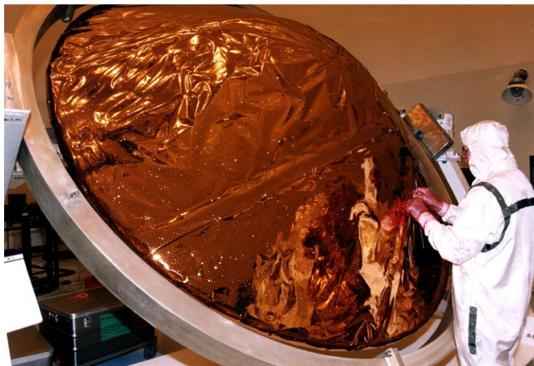
Figure 3-6: Multi-Layer Insulation covering the Huygens lander [194]. Highly reflective surfaces such as these are common on spacecraft and can cause intensive light reflections and glare, as well as hide spacecraft structural features important for relative navigation.
