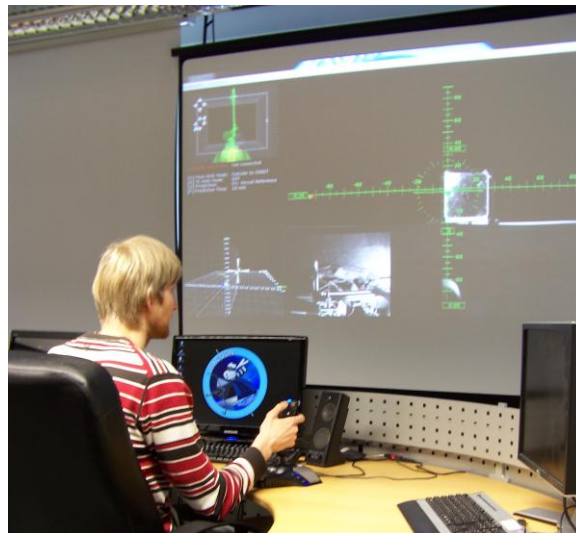
Figure 5-3: Operator sitting at his workstation. The main output is displayed by a video projector. The small monitor is used for auxiliary data. The main input devices are keyboard, joystick and space mouse, which are interfaced by a custom-built computer program.
