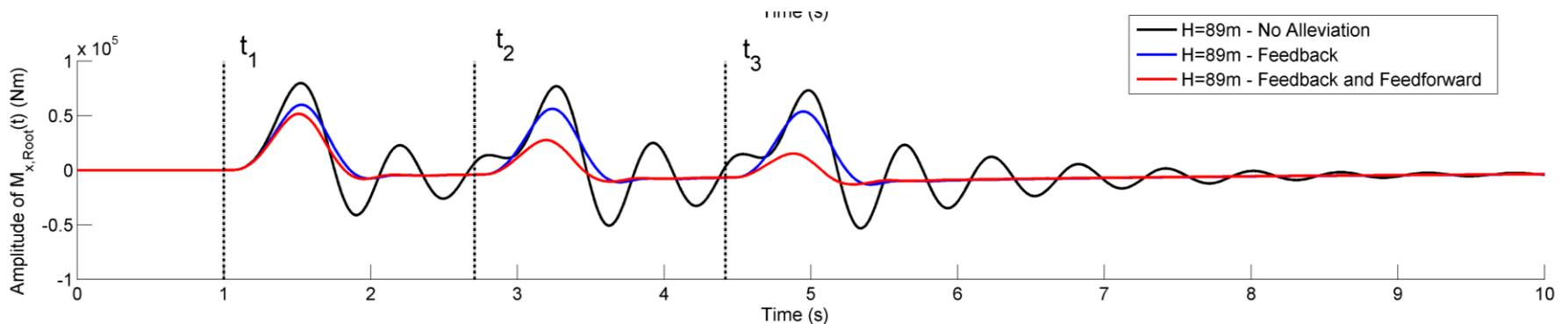
→ Peak reduction increases with time, as filter parameters are adapted
