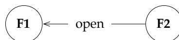
Figure 2.14.: Feature interaction example: if F2 gets activated, the window is forced to open.
