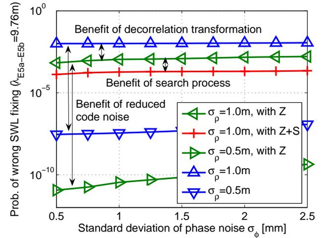
**Fig. 1** First step of CIR: Fixing of SWL ambiguities for worst-case geometry and variable code noise
