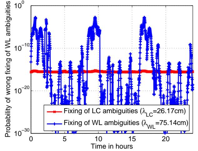
**Fig. 5** Second step of CIR: Time dependency of probability of wrong fixing for different widelane combinations
