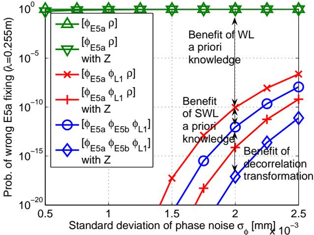
**Fig. 3** Third step of CIR: Fixing of E5a ambiguities for worst-case geometry and code noise  $\sigma_\rho = 1\text{m}$
