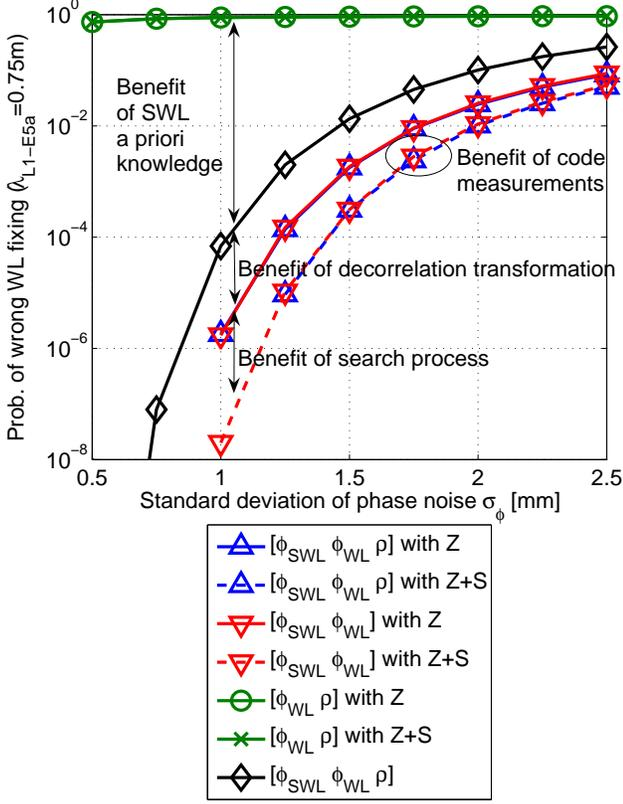
**Fig. 2** Second step of CIR: Fixing of WL ambiguities for worst-case geometry and code noise  $\sigma_\rho = 1\text{m}$
