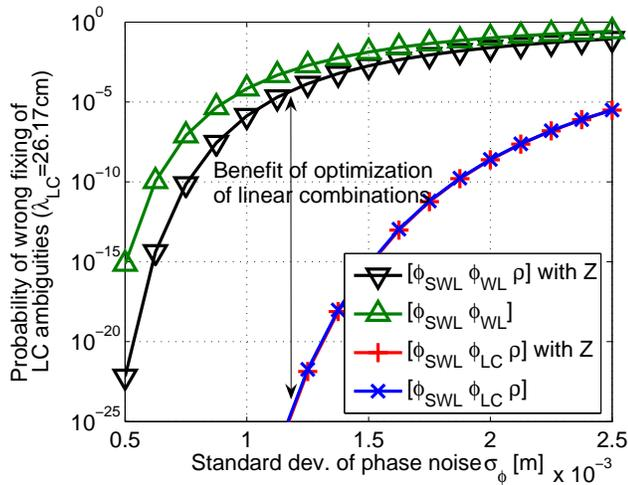
**Fig. 4** Optimization of linear widelane combinations for 2nd step of CIR: Weighting  $[-3, 38, -34]$  of  $L_1$ ,  $E_{5b}$  and  $E_{5a}$  integer ambiguities
