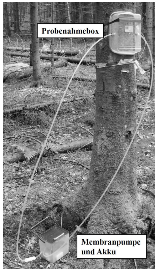
Abb. 10: Mobiles Closed-Loop VOC-Sammelsystem
