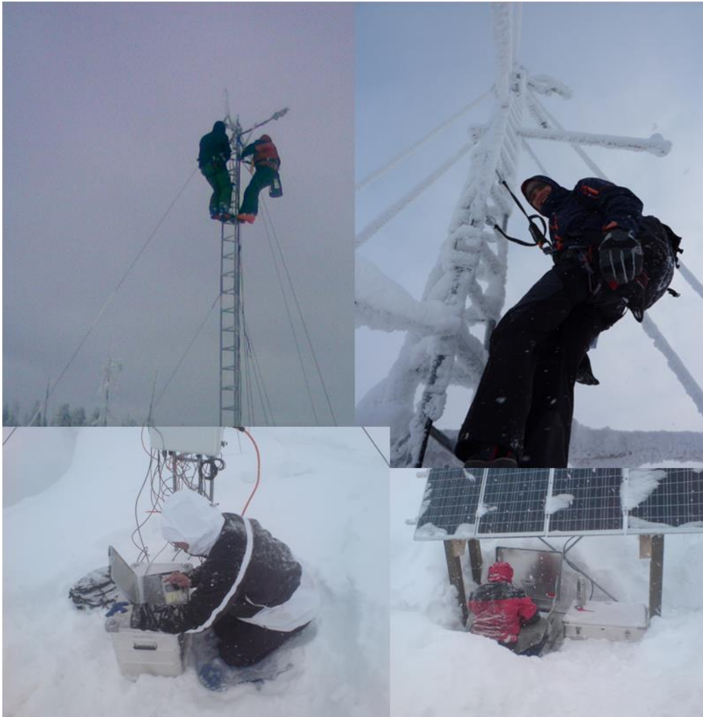
Figure 18. Instrumentation of the central station Lackenberg, 16.-20.02.2009. Clockwise from the upper left corner: Installation of the eddy covariance system (with Rainer Steinbrecher); an example for data loss due to riming of sensors; installation of the power supply (Carsten Jahn); data collection (Matthias Mauder).
