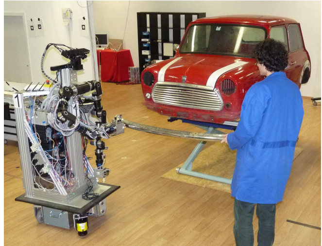
Fig. 1. Experimental scenario: Human and robot jointly carrying a bulky bumper to its mounting location during car restoration.
