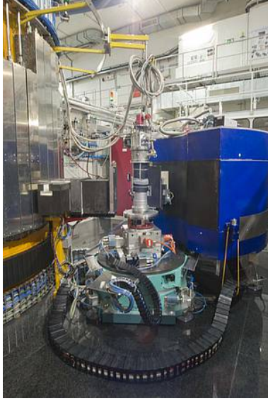
Figure 3.5: Photo of the PUMA instrument at Forschungs-Neutronenquelle Heinz Maier-Leibnitz (FRM II). Yellow drum shows the monochromator shielding, gray cryostat shows the sample position with sample environment and blue drum shows the analyzer shielding. Taken from http://www.frm2.tum.de/de/wissenschaftliche-nutzung/spektrometrie/puma/index.html
