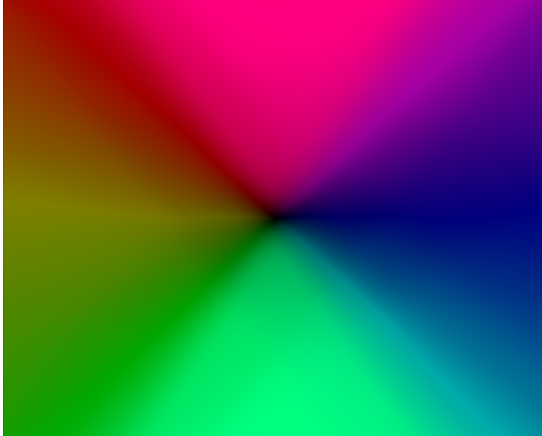
Figure 4.8: Gradient direction (encoded by color) and magnitude (encoded by brightness) for the line fitting problem when using the Pseudo-Huber cost function. Comparison with Figure 4.10 reveals a high degree of similarity to the “ideal” behaviour with respect to convexity.
