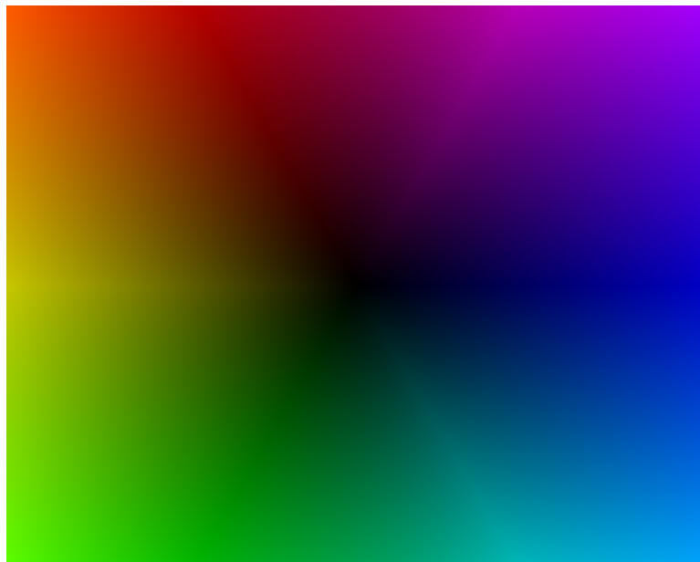
Figure 4.10: Gradient direction and magnitude for a hypothetical cost function that would be optimal in the sense that every gradient points towards the minimum located at the center, and that gradient magnitude becomes smaller as the minimum is approached.
