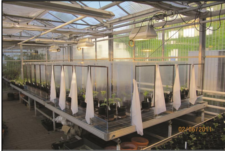
Figure S1: The Plexiglas cages (35L×35W×90H cm) which used for the experiments in the greenhouse in order to prevent the escape of aphids. To facilitate air ventilation, the front of the cages was covered by fine mesh.
