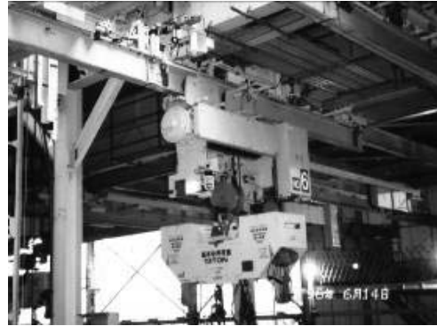
Construction adapted and highly specialized OM used in on-site factories in construction, Shimizu, Japan
