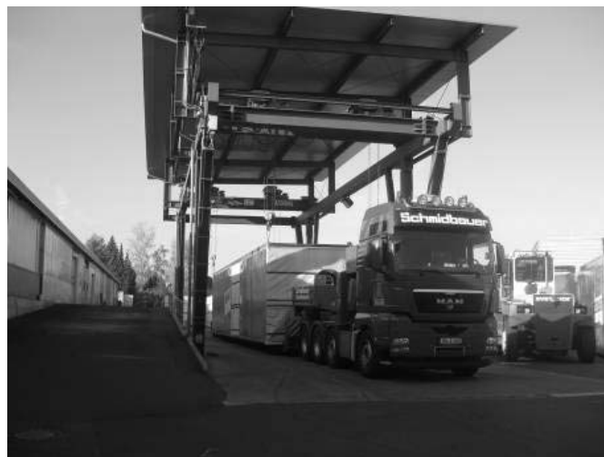
Figure 6-6: station for loading large sized units onto special transport trucks. Cadolto, 2011. (Picture Source: Linner)
