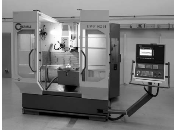
Advanced computer controlled reprogrammable machining center with more than 4 DOFs
