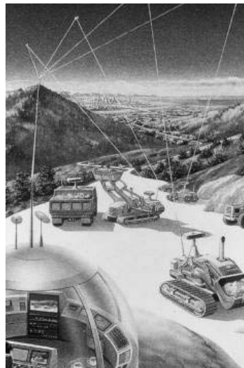
Figure 4-9: Multiple cooperating construction robots are operated by a single human supervisor from a central box, Vision Sketch (picture courtesy of Japanese Research Institute, 1980 )
