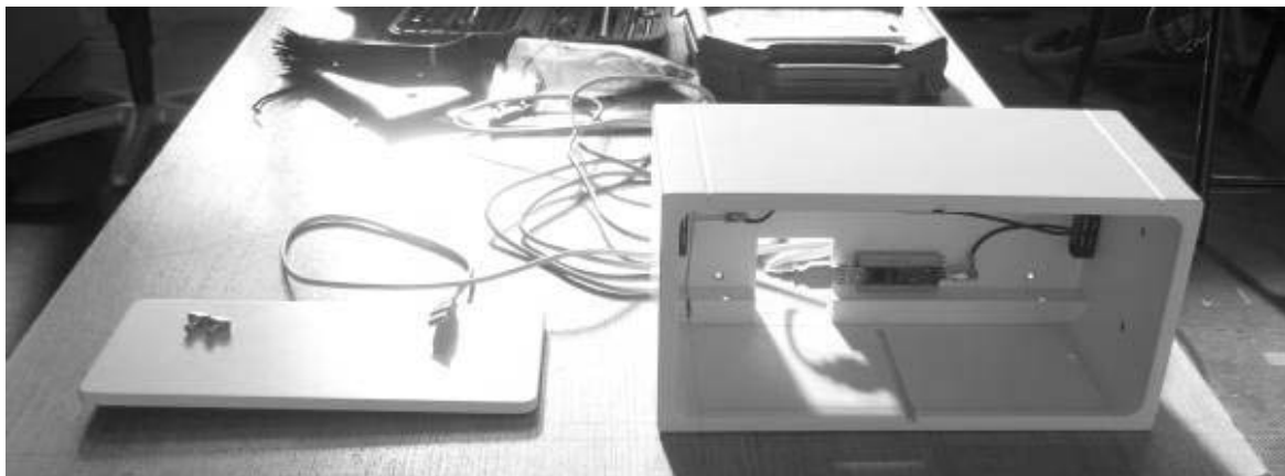
Figure 2-8: Shows a cabinet with removed top plate and sensor infill (system for reading multiple RFID-tags). Each cabinet, and thus its sensor system infill, is connected to the basic wall unit (which also integrates a mini server as “brain”) by a USB connector. USB provides electricity as well as data transfer capability. Connector system developed by the author within LISA.
