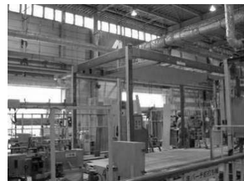
Automated sending of 3-D space frame along assembly line
