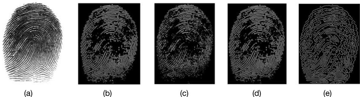
Figure (1.16): (a) Finger print image, (b) Edges image by 3*3 Prewitt edge detector, (c) Edges image by 2*2 Roberts detector, (d) Edges image by 3*3 Sobel detector, and (e) Edges image by Canny detector with filter size of 1.5
