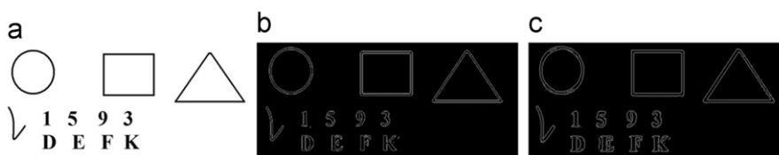
Fig. 10. (a) Gray level image with primitive features, and its edges image produced by the proposed method (mask size= 5 \times 5 , flux check matrix size= 3 \times 3 , w=0.75 ) with a mask represented pixel set at (b) mask centroid, and (c) mask center.
