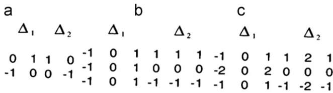
Fig. 2. Basic gradient operators for (a) Roberts, (b) Prewitt, and (c) Sobel edge detectors. \Delta_1 is the gradient operator in x direction, while \Delta_2 is in y direction.
