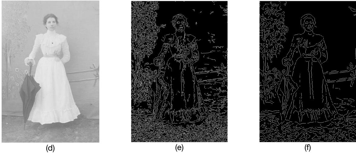
Figure (2.24): Canny detector outputs for two grey scale images indexed by (a) and (d). (b) and (e) are the edges images when \sigma = 1 , while (c) and (f) the edges images when \sigma = 2 .
