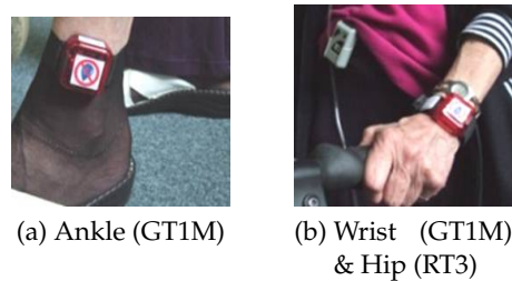
Figure II-5. Accelerometer measurement positions in patients suffering from COPD
