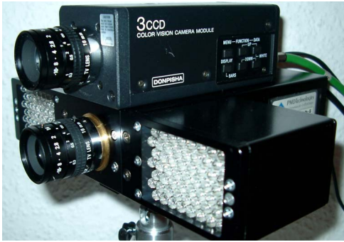
Fig. 2. Piggyback assembly of PMD and color CCD.
