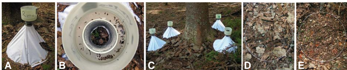
Fig. 3.6. Setup of soil emergence traps. A. Trap consisting of a wire skeleton, a reversed cloth funnel and a container on top. B. Close-up view of the top container containing preservation fluid (ethylene glycol/water, 50% v/v) and soil emerged beetles. C. Trap pairs at the base of trees with more than 50% fallen bark. Below one trap of each pair the fallen bark was D. left and E. removed.
