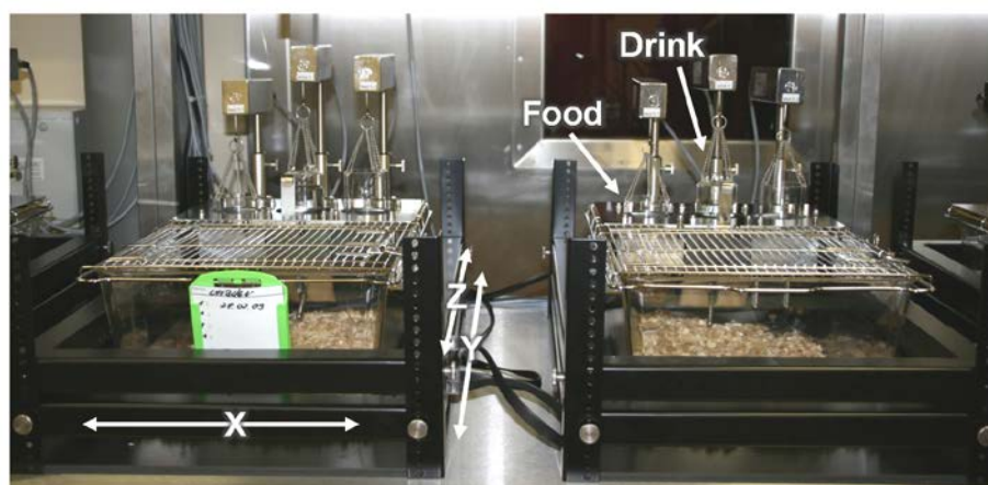
Fig. 2-1. Feeding-drinking-activity system. Individual cages are surrounded by sensor frames containing emitter and receiver diodes. Diodes of the Z-frame are located above the Y-frame. Counts of beam breaks of the X- and Y-frame constitute horizontal activity, counts of beam breaks of the Z-frame refer to rearing activity. Food was supplied in one basket.
