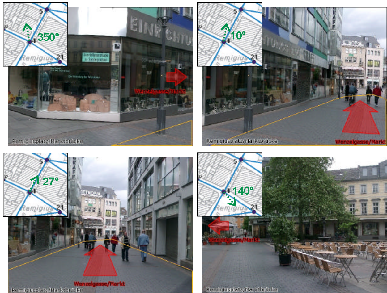
Figure 8: Visualization of virtual signposts in different viewing directions at the same location.
