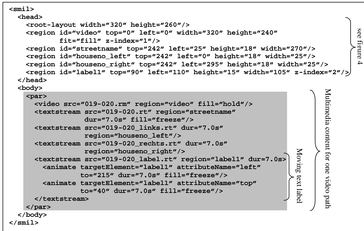
Figure 3: Example for the definition of a multimedia clip for one directed walking path using SMIL 2.0. The head section defines the screen layout for the different media elements. Please note, that “labell1” lies in the same area as “video”, but is shown on top due to a higher z-index . The body element references and synchronizes five media elements: the walkthrough video clip, the street name, the current house numbers on both sides, and a text label.
