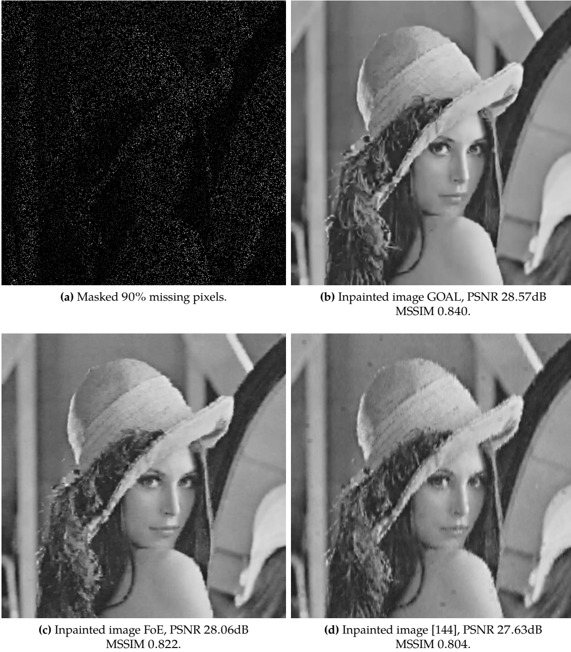
Figure 5.8: This figure shows the achieved results for filling up missing pixels of the "lena" image from 10% of all pixels using \Omega^* learned by GOAL (b), FoE (c), and [144] (d).
