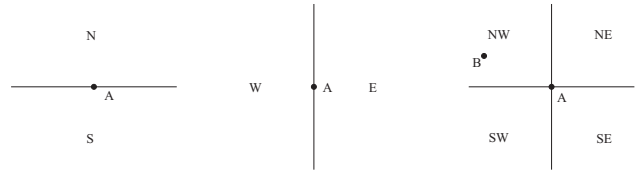
Fig. 3. The projection-based model for point-shaped objects in 2D [33]. The space is dissected horizontally (left) and vertically (right), then the resulting halfspaces are superimposed, thus creating 4 space partitions.
