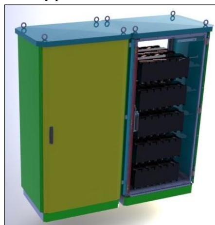
Fig. 6: CAD design of the 2 nd -life battery pack
