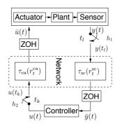
Fig. 1. Illustration of NCS over communication network, the transmission delay from sensor-to-controller  $\tau_{\rm sc}(r_t^{\rm sc})$  and from controller-to-actuator  $\tau_{\rm ca}(r_t^{\rm ca})$ .
