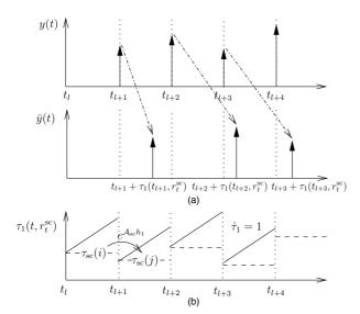
Fig. 2. The sampled output measurement y(t),  $\bar{y}(t)$  (a) and the evolution of time delay  $\tau_1(t, r_t^{\rm sc})$  for certain sample path of  $\tau_{\rm sc}(r_t^{\rm sc})$  (b).
