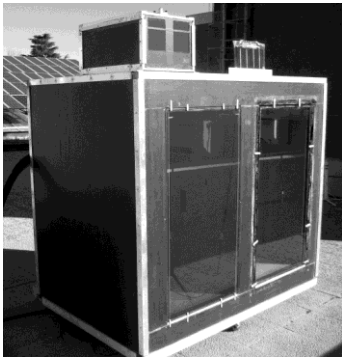
Figure 1. West and south views of the testing facility. The STPV module is installed on frontal side of the left box. On the frontal face of the right box a code-compliant glass is mounted. On the upper face the scale model used in the daylighting tests and the reference solar cell are installed.
