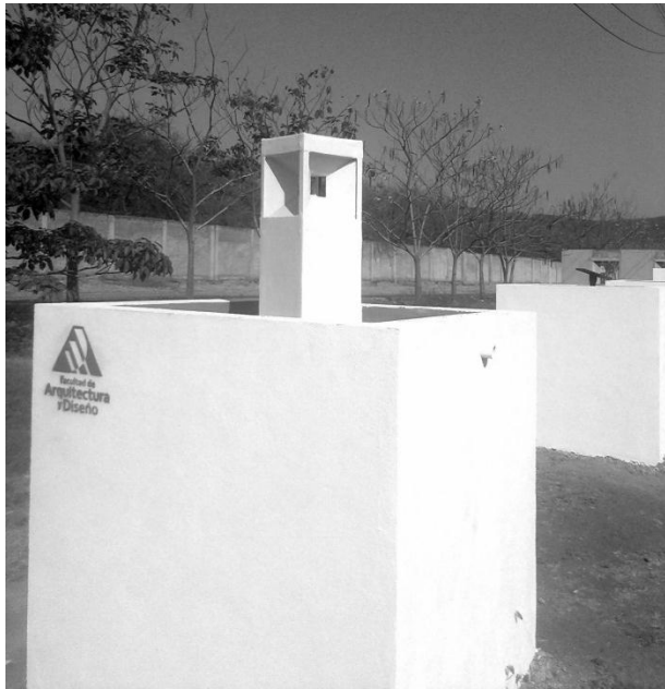
Figure 6. Wind tower model installed on experimental module. Source: Authors
