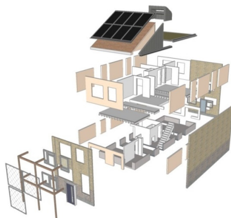
Figure 7: Exploded view highlighting component kit
