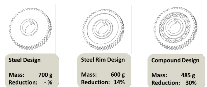
Figure 2: Mass reduction for gears with different design options
