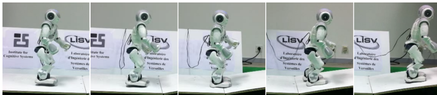
(b) Walking from flat ground to upward slope with switching between success maps neurons.
