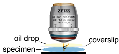
Figure 9: Physical representation of the numerical aperture, which relates to the amount of light that can be captured by the objective. Increasing the half angle \alpha and the index of refraction \eta between the objective and the coverslip will serve to maximise NA. Note in the inverted configuration as used in our own experiments, the objective sits below the sample (coverslip faced downwards).
