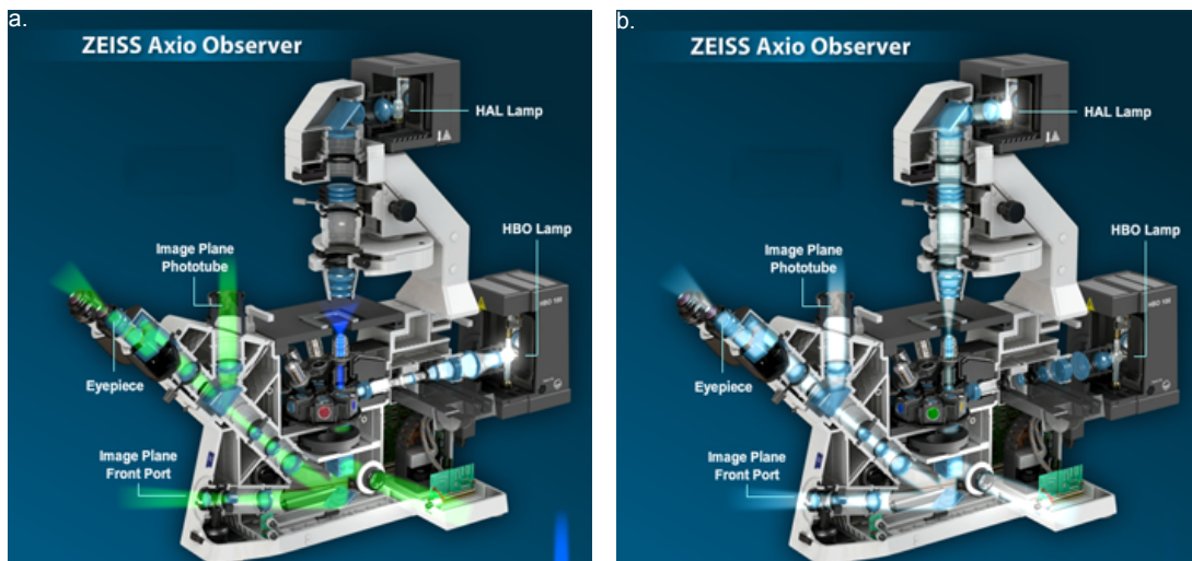
Figure 6: Schematic of a Zeiss inverted fluorescent microscope with the corresponding optical path. a. Epi-fluorescence mode modified from [107]. The optical train in reflected mode is shown originating from the Mercury arc lamp (HBO), where, after passing through the filter blue light, excites the sample so that green light emission is reflected back to the eyepiece appropriately separated from the blue excitation light. b. The optical train of transmission mode originates from the tungsten halogen lamp (HAL), illuminating the sample, whereby a significant portion of the excitation light remains with the emission light. Note the absence of the filter cube in the transmission mode.
