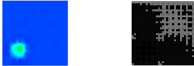
Figure D.1.: Reconstructed control and adaptively refined mesh for the linearized version of Example 3 (a)(i), 1% noise, f = f_1 , Neumann zero boundary conditions
