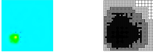
Figure D.3.: Reconstructed control and adaptively refined mesh for the linearized version of Example 3 (a)(i), 1% noise, f = f_2 , Dirichlet zero boundary conditions
