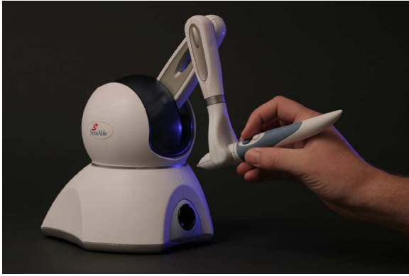
Fig. 9. The SensAble Phantom Omni device used for the experiments [http://www.sensable.com].
