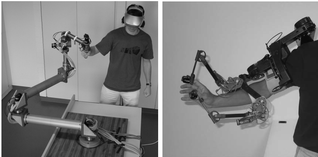
(a) Non-portable kinesthetic interface: VISHARD 6 [12]. Reprinted, with permission, from M. Ueberle and M. Buss, Design, control, and evaluation of a new 6 dof haptic device, IROS, 2002 (b) Portable kinesthetic interface [10]. Reprinted, with permission, from V. Hayward, O. R. Astley, M. Cruz-Hernandez, D. Grant, and G. Robles-De-La-Torre, Haptic interfaces and devices, Sensor Review, 2004
