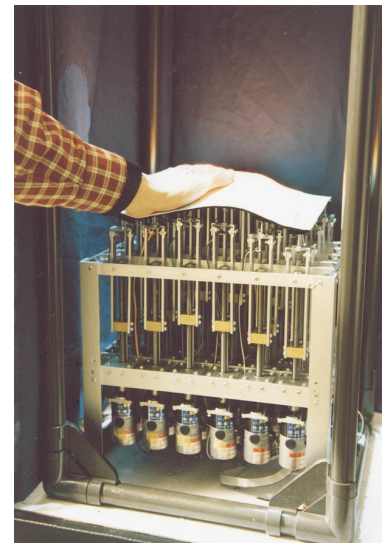
(b) FEELEX 1: pin array, actuated [21]. Reprinted, with permission, from H. Iwata, H. Yano, F. Nakaizumi, and R. Kawamura, Project FEELEX: adding haptic surface to graphics, Computer graphics and interactive techniques, 2001
