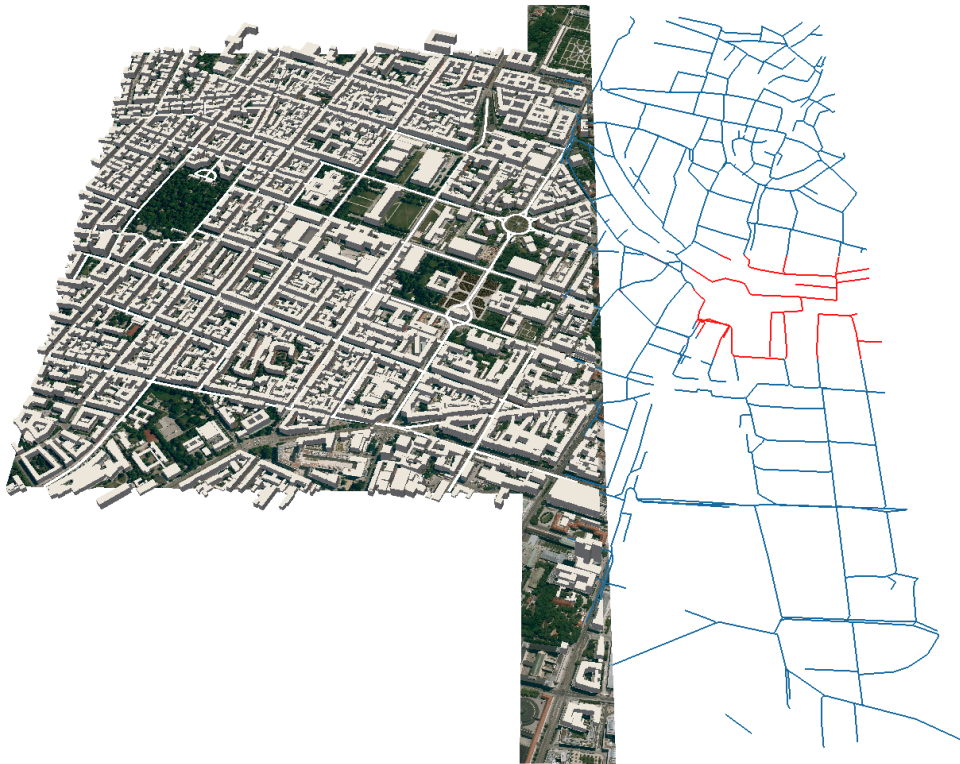
Figure 4.21: The evaluation of possible intersections of a sewer network with existing constructions in the city is performed by deriving the hierarchical representation of both configurations.
