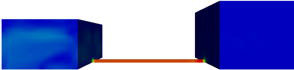
Figure 7.3: A three-dimensional benchmark of two basins connected with a pipe implies that resolving the pipe with a single voxel in the orthogonal directions of the flow imposes the characteristic of one-dimensional flow.
