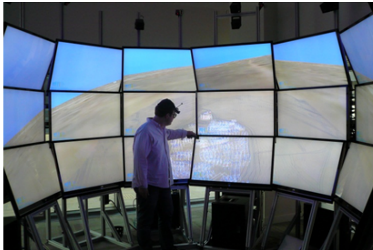
Figure 4.18: The position and direction of the user's view is derived from the tracked marker mounted on their head. From this information the viewport and thus the projection onto the different planes of the CAVE are derived, here for the NEXcave@KAUST.
