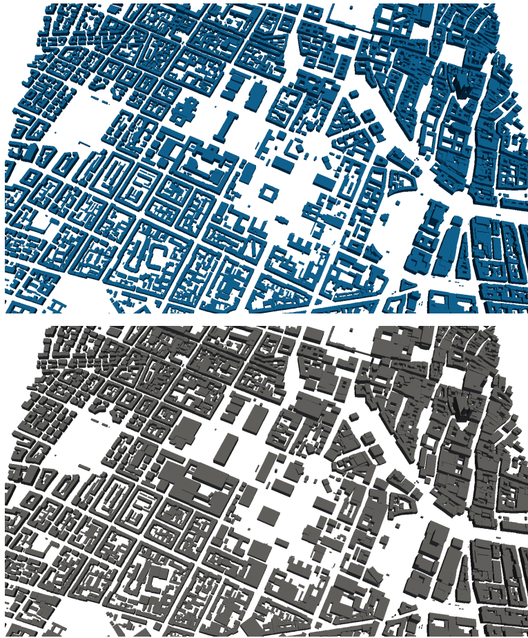
Figure A.1: The city model of city centre Munich spans an area of 2.8km by 2.3km. For the single polygonal building descriptions (top) the aligned bounding boxes are calculated (bottom).
