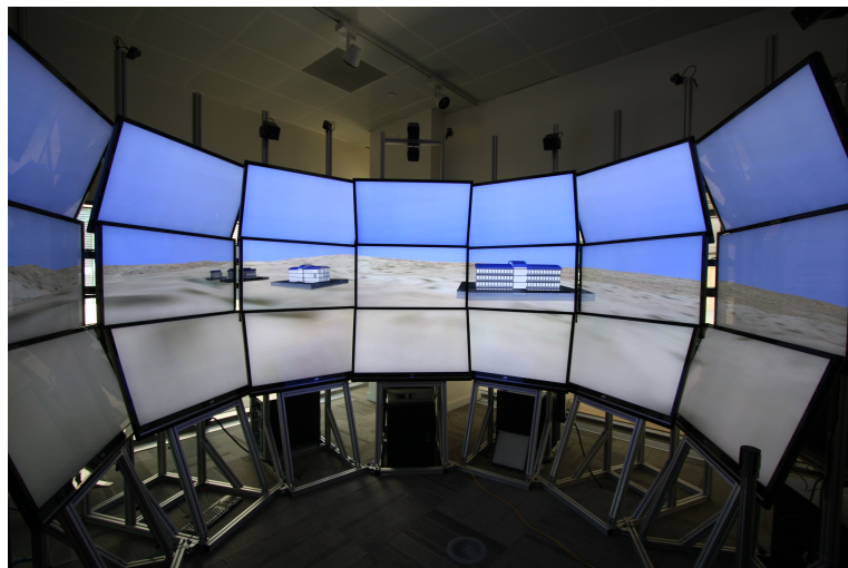
Figure 4.13: On the NEXcave@KAUST the visualisation of fully detailed product model data on a local scale is performed by rendering the outer shell of the constructions on 21 monitors.
