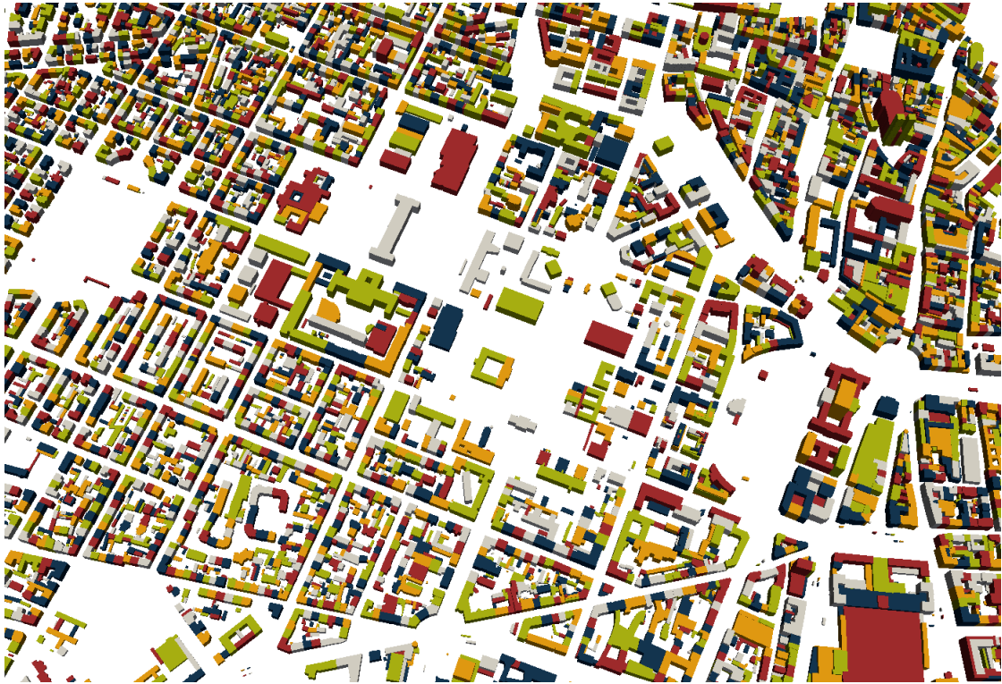
Figure 3.7: Based on a given mapping of m product models to n processors, the colour indicates the distribution of the models over the processors. All models of a processor are depicted with the same colour.
