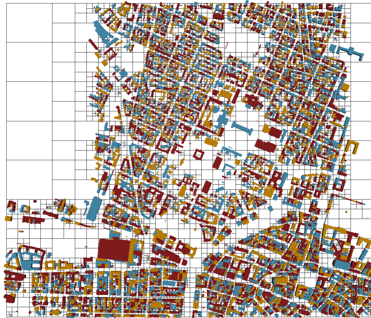
Figure 3.14: The quadtree representation of the product models is generated on the basis of the centre points of their bounding boxes projected along the z-axis.
