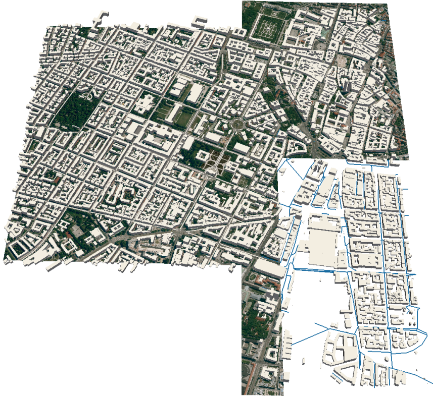
Figure A.3: For Munich city centre, a city model data set is created which fuses the specification of the terrain with its texture, the building assembly and the underground water drainage system.
