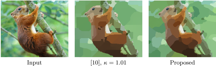
Fig. 8. Grid artifacts of L_0 -Smoothing [10]. The method [10] (center, \lambda = 0.035 ) measures edge lengths with the anisotropic l^1 -norm. This leads to significant artifacts as result edges tend to align with coordinate axes. We use the l^2 -norm (right, \lambda = 0.82 , \alpha = \infty ), yielding more natural results.
