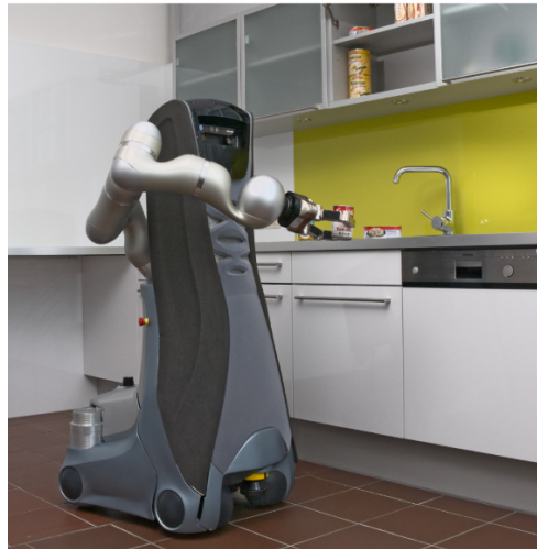
Fig. 3.39: Our mobile robot equipped with three laser scanners, a Kinect camera and a stereo camera system.
