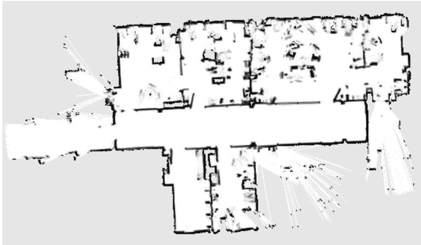
Fig. 3.1: A typical occupancy grid map of an indoor environment, obtained from the Robotics Data Set Repository (Radish) [58].
