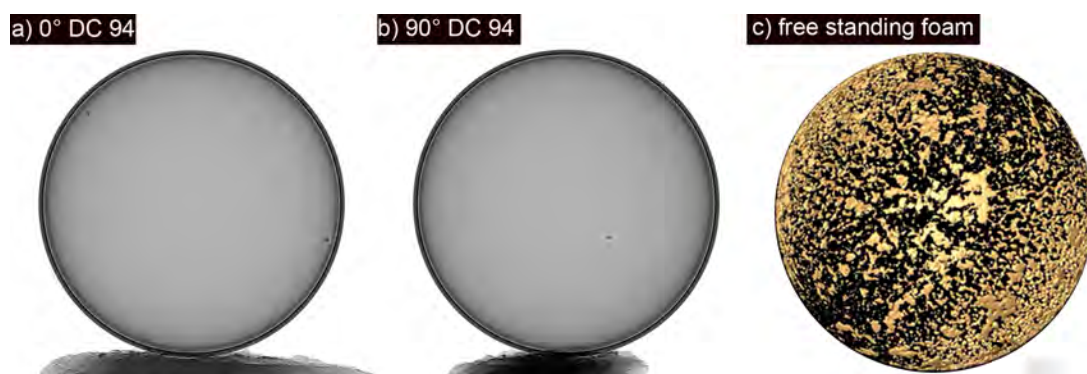
Figure 5.36: Capsules with a dried foam layer - a-b) show diamond capsule 94 after drying and doping with iodine. The layer is almost uniform. c) the free standing film with the diamond capsule removed shows a band with less coating. This coating was pure PDCPD without the addition of NB
