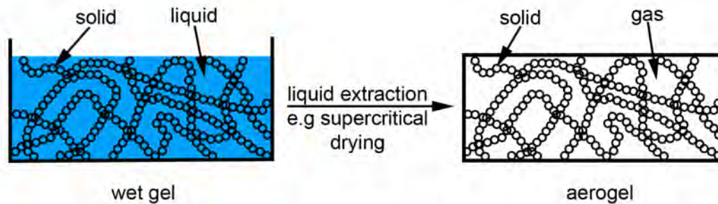
Figure 1.4: Aerogel schematic - particles form a chain within a liquid which is usually done by a catalyst or condensation reaction. The liquid is then removed by supercritical drying or freeze drying leaving particle chains behind. The shape of the dried gel has the same shape as the liquid gel had before
