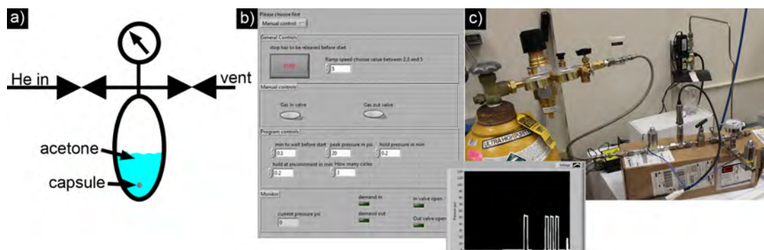
Figure 5.31: Pressure cycling setup - a) shows the schematic pressure cycling setup where the pressure within the pressure vessel is controlled by two valves; b) the lab view interface to control the pressure setup with an exemplary pressure curve on the lower right; c) the actual setup build with VCR fittings and tubing
