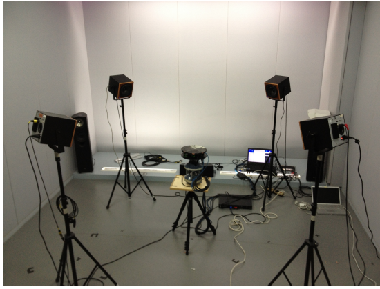
Figure 5.1.: Recording setting of the channel assignment experiment in the echoic environment
