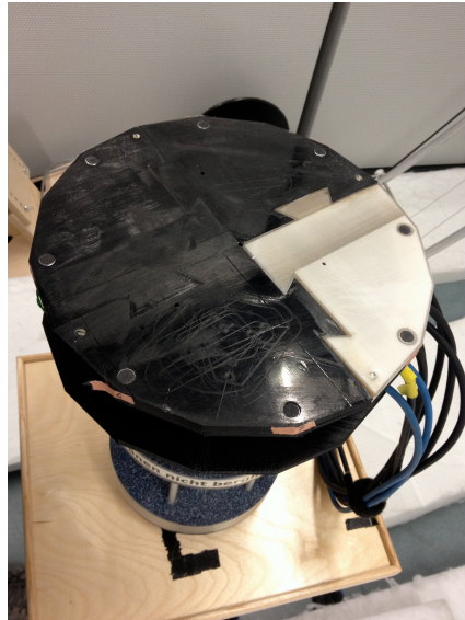
Figure 2.1.: Microphone Array 1: The planar shape of the array is constructed with respect to the SRP-PHAT algorithm
