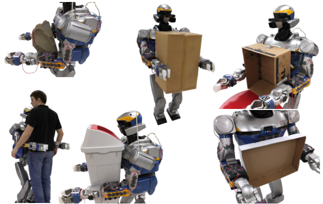
Fig. 1. A position controlled HRP-2 humanoid, holding unknown objects with the whole body, as result of a multi-modal tactile grasping sequence.
