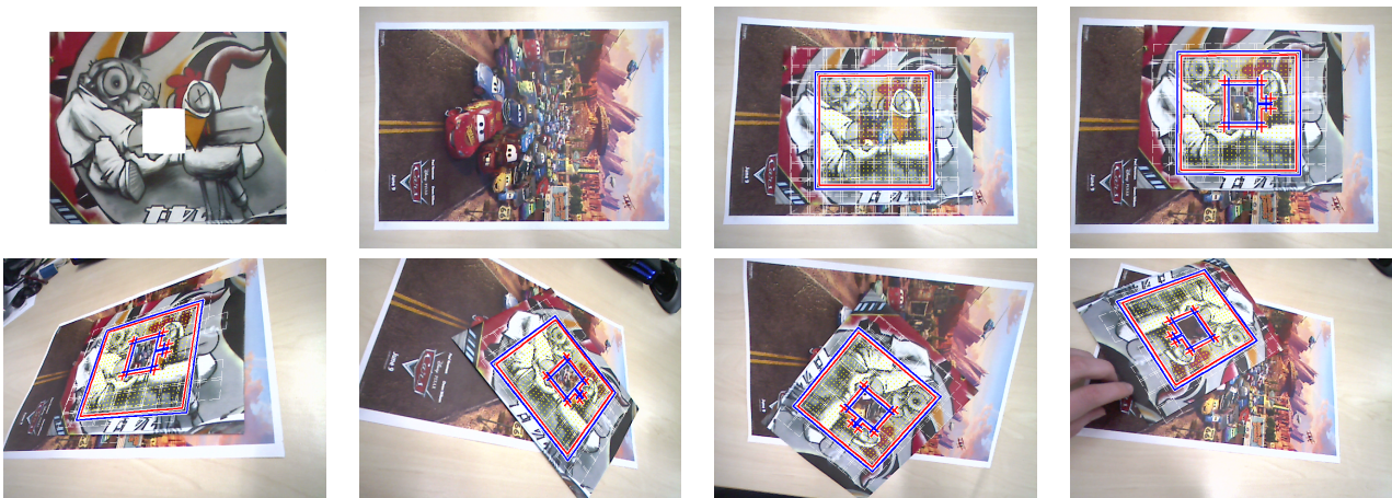
Fig. 17. Tracking a template with a hole inside. The first image shows the template on a white background to show the hole in the middle. The second image shows the background. In the right image the template is learned with the background image. In the remaining images the template tracking results are shown. Note that the background behind the hole is changing, thus the hole is removed from the template and does not disturb the tracking.
