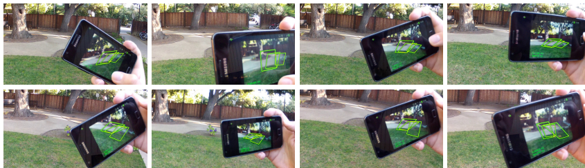
Fig. 9. Tracking of multiple templates on a mobile phone. The most right template shown in the first row failed during tracking and was replaced by a new template in the second row.
