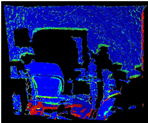
Fig. 7. Visualization of the difference between the normals estimated using our covariance matrix approach and the approach of [17]. For every point in the point cloud we visualize the dot-product between the normals estimated with the different methods, where blue color corresponds to a small and red corresponds to a large difference between the normals.
