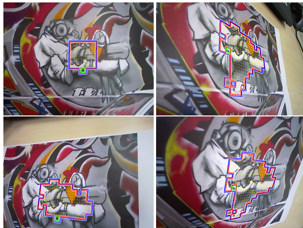
Figure 1. An initial small template is enlarged according to a tracking quality measure. The template is tracked over time and reduced if parts of it go out of the image. The removed parts are reinserted as soon as they become visible.
