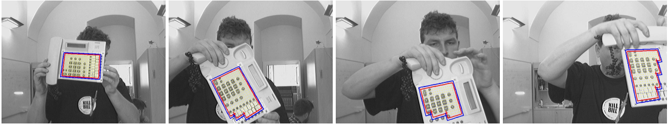
Figure 8. Result images of the phone sequence, which is provided by Zimmermann et al. [20]. Note that the template is reduced if it goes out of the image and grown again if it gets visible again.
