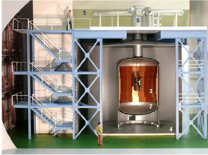
Figure 2.1: Cutaway view of the GERDA experiment (Ge array not to scale), showing the main hardware components: the germanium detector array (1); the LAr cryostat (2) with its internal copper shield (3) and the surrounding water tank (4) housing the Cherenkov muon veto; the GERDA building with the superstructure supporting the clean room (5) and the lock (6). Various laboratories behind the staircase include the water plant and a radon monitor, control rooms, cryogenic infrastructure and the electronics for the muon veto. Taken from [19].
