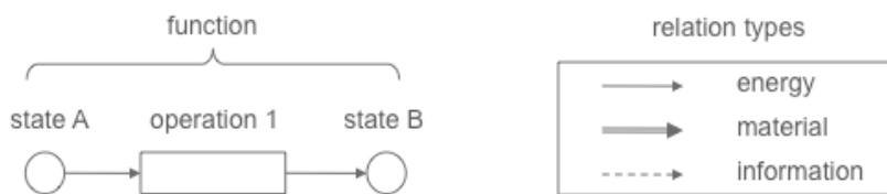
Figure 5-15 Semantics of the flow-oriented functional model [according to EHRENSPIEL 2009, p. 398, PONN & LINDEMANN 2008, pp. 64-66]
