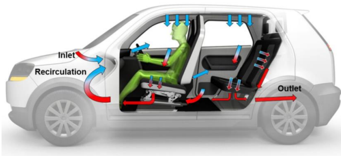
Figure 9: Air distribution in EVA interior
