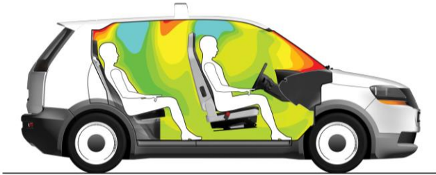
Figure 8: Temperature layering in individual climate zones inside the cabin
