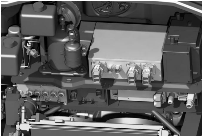
Fig. 4. Front compartment with HV, LV and cooling components.
