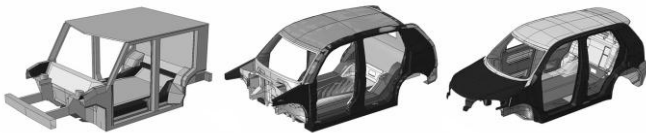
Fig. 5. FLTR: H0, H1, H2 the development phases of the vehicle structure.
