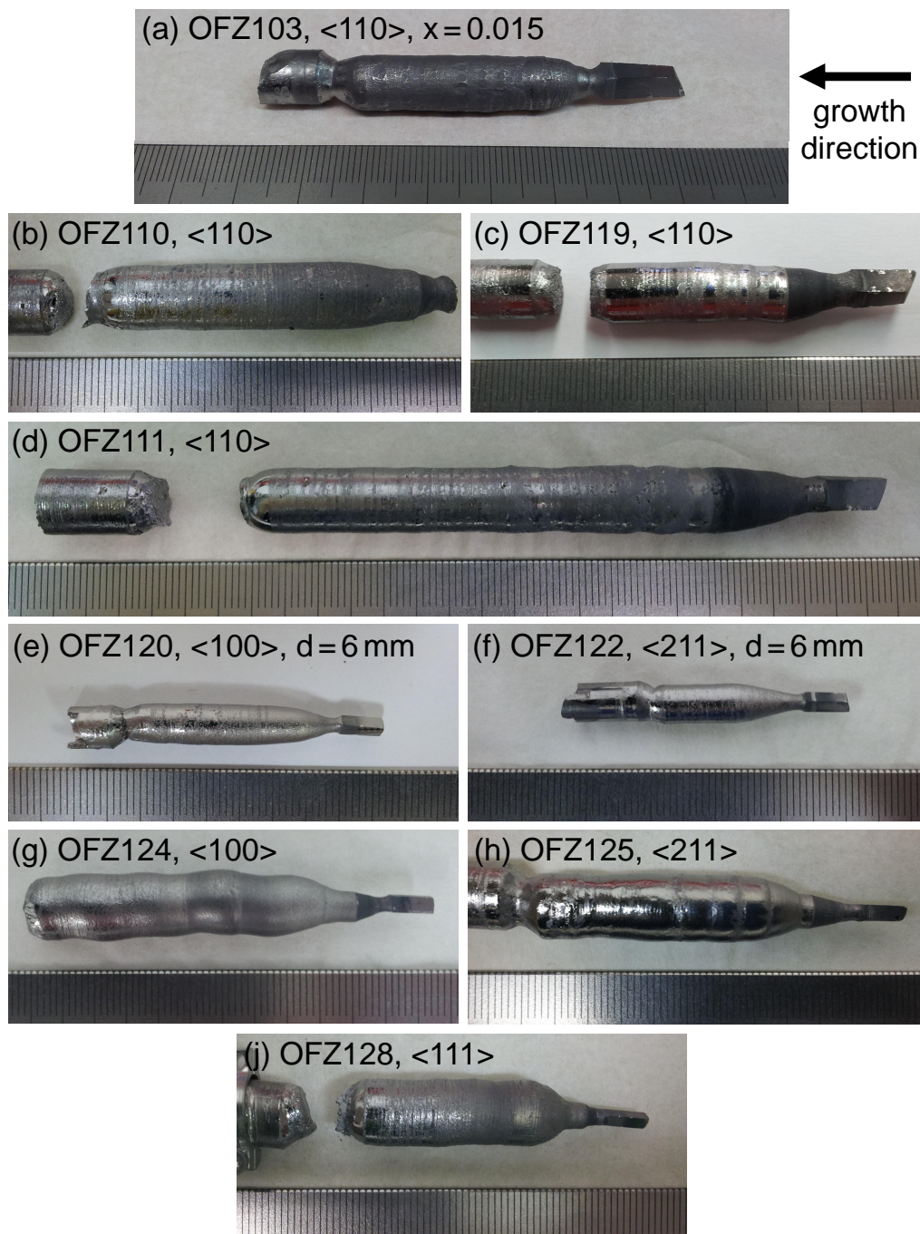
Figure 3.25: Float-zoned single crystals of MnSi with major crystallographic directions along their axes. Oriented single crystals were used as seeds. All scales are in millimeter.
