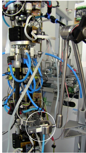
Figure 6.8: Setup for force/torque test with load cell – discrete case
