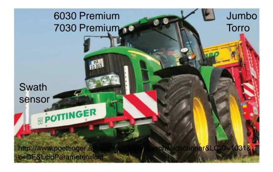
Initiated by the Implement-ECU the tractor speed is modified depending from rotor torque and incoming swath size
